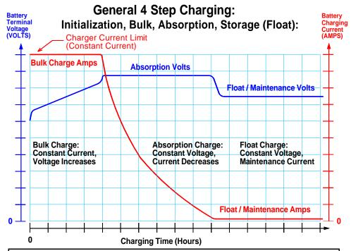
**Step 1) Initialization:** Red Light On, Green Light off: Monitor Circuit verifies appropriate battery voltage levels and good electrical continuity between the battery and the charger DC output.
