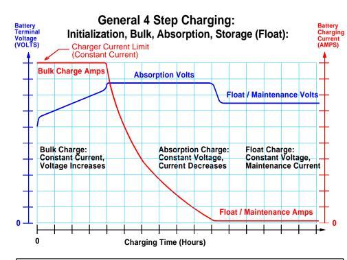
**Step 1) Initialization:** Yellow Light On or Yellow Light Flashing: Monitor Circuit verifies appropriate battery voltage levels and good electrical continuity between the battery and the charger DC output.
