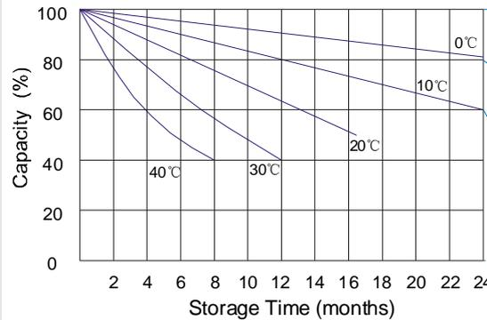
Supplementary charge required (Carry out supplementary charge before use if 100% capacity is required)
